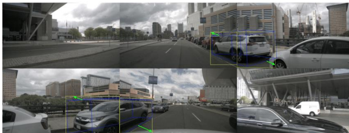
(b) The detection results of SimPB. The process of 3D-to-2D association (green arrow) effectively yields accurate 3D results along with their corresponding 2D boxes for cross-camera targets.
