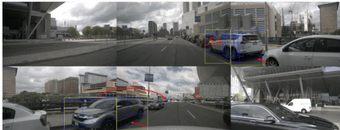
(a) The detection results of MV2D. 2D-to-3D association (red arrow) may produce duplicate 3D results or unrelated results from 2D priors for a cross-camera target.
